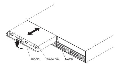
Figure 40. Removing and replacing a controller
